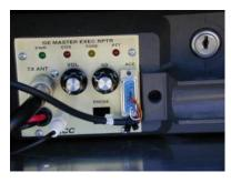
Discovered no discriminator audio present on the MCC accessory connector pin 11 (DB15). There was "Receiver Audio Output" on pin 2, but with de-emphasis filtering. We decided to use this connection but only until we could figure out why there was no discriminator audio at pin 11. The pin out of the DB15, as indicated on MCC's document is:
