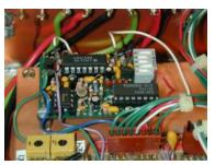
This was a simple modification, and the setting the CTCSS encode level was easy once the controller was re-installed into the rack. Then set the CTCSS TX deviation to 1 kHz, and the repeat audio deviation at 5 kHz. Tested for CTCSS functionality with my handy talky and my mobile rig. All worked fine.
